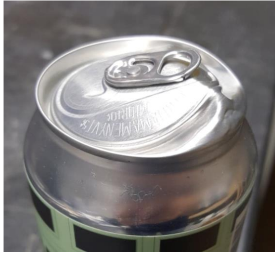
Figure 7: Can from the second canning batch that experienced over-pressurization. This can was held at room temperature.
