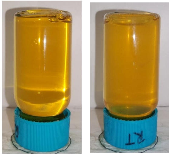
Figure 16. Side-by-side comparison of the refrigerated (LEFT) and room temperature (RIGHT) for the beer aged for 67 days. There is an observed difference in the haziness between the two samples.
