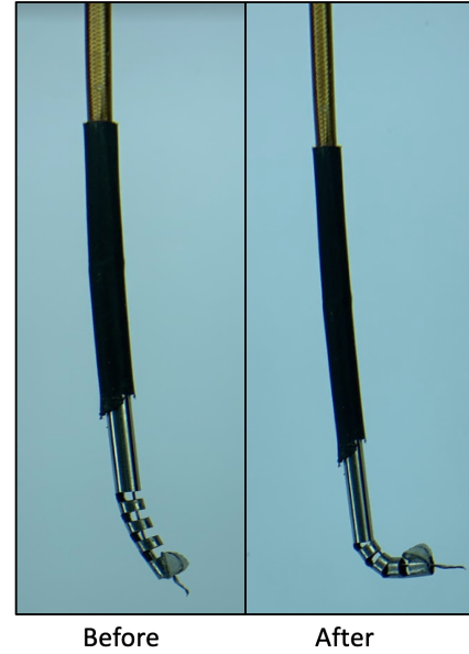
Figure 26: Bending of notched tube by 90 degrees
