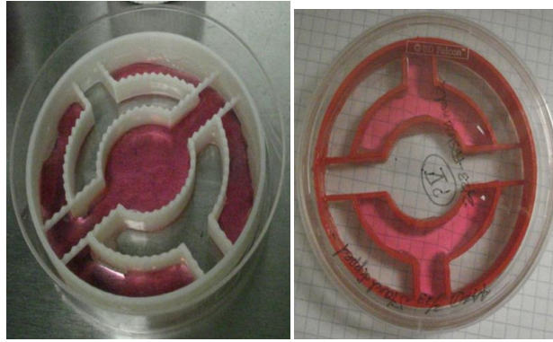
Figure 27: Fluid-filled wells illustrating the different well sections within the radial-well ring device
