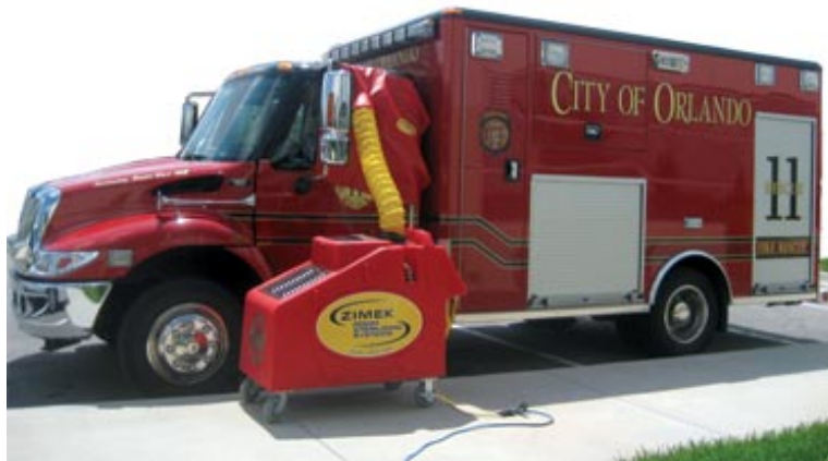
Figure 26: A ZIMEK Micro Particle Disinfecting System in Operation
