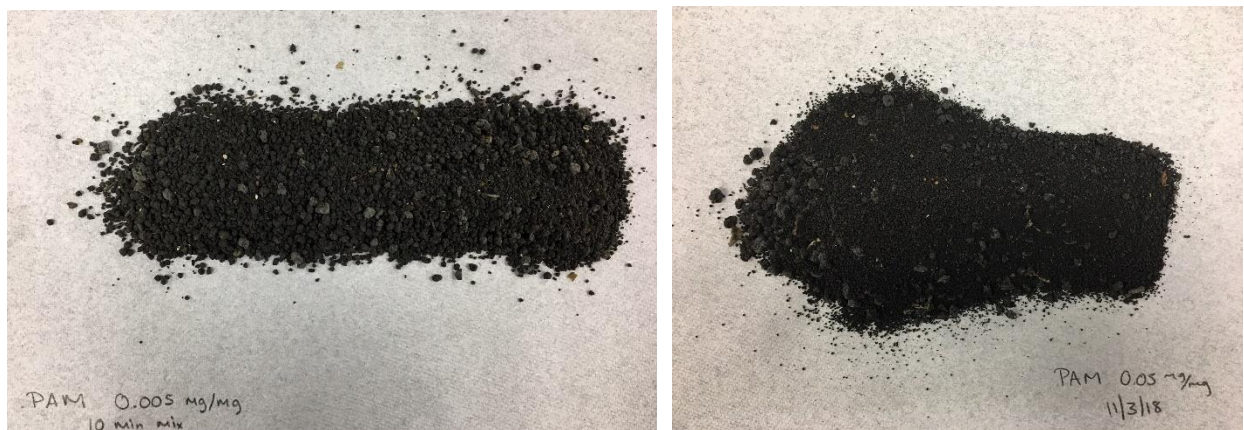
Figure 18 - Photos of Pellets Dried with PAM
