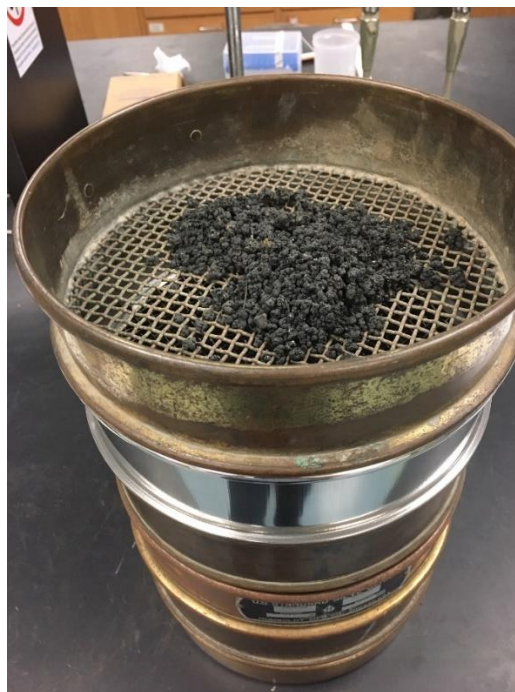
Figure 13 - Sieves for Pellet Size Analysis
