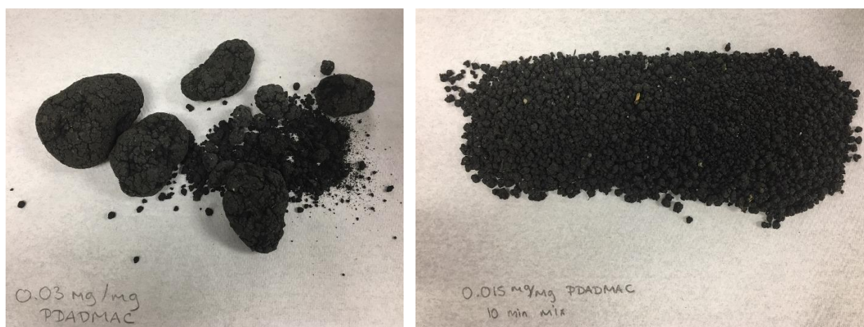
Figure 15 - Photos of Pellets Dried with PDADMAC at Varying Concentrations
