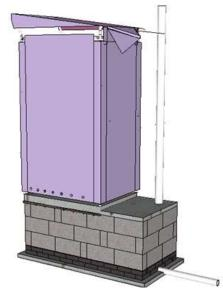
GSAP Microflush (GMF) toilets are environmentally friendly latrines that combine two main technologies: a filtered digester bed and the titular Microflush valve. The valve was developed by the S-Lab of Providence College. It uses a "pour flush" model where the previous user's handwashing water cleans the valve and flushes the waste through the aforementioned filtration layers.
