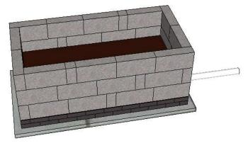
• Must demonstrate the proper block layout & include visible mortar, still be empty aside from plastic mesh
