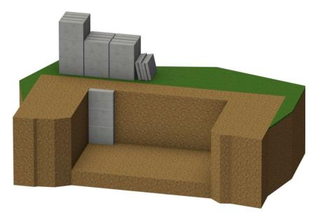
6. Pour a layer of gravel at the bottom of hole, remove sticks & rope
