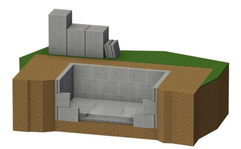
9. Lay Plastic Mesh layer on top of blocks
