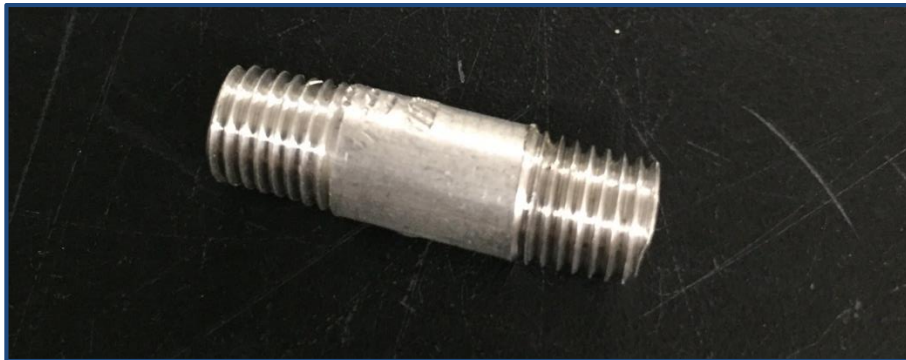
Figure 38: Threaded Crankshaft Link
