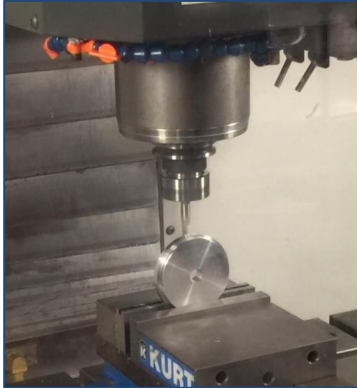
Figure 29: Piston Pin Holes cut in the VM2
