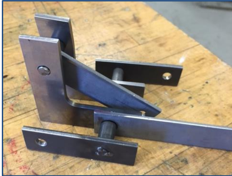
Figure 42: Constructing the Crank
