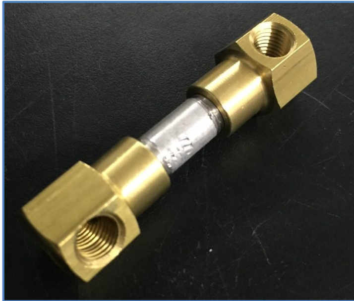
Figure 39: Misaligned Threading & Connectors
