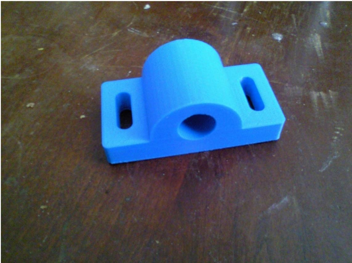
Figure 18: 3D Printed Bushing
