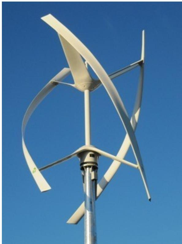
Figure 3: Standard Vertical-Axis Wind Turbine
