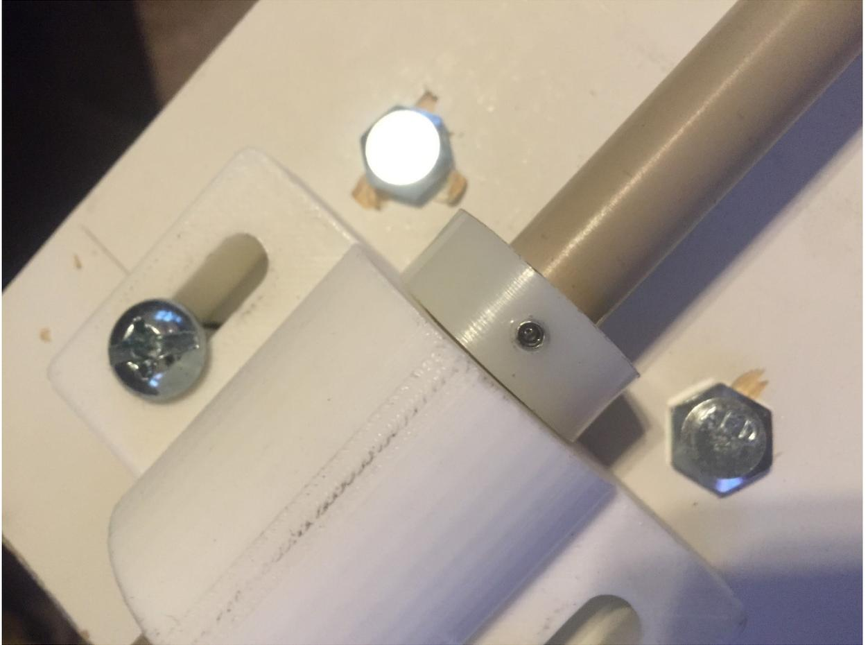
Figure 19: Nylon Washer with Locknut
