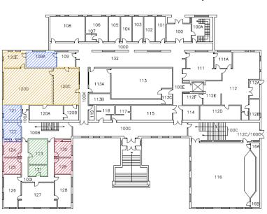
The example map (above left) that was generated from the LiDAR and IMU module is compared to an actual floor map of the same area (above right). The system uses Hector SLAM for mapping and localization, which can also be achieved using the Microsoft Kinect.
