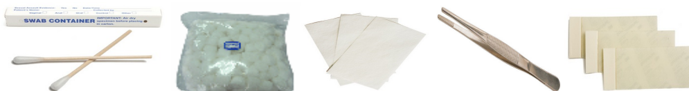
Figure 23: Common collection media used in sample collection. From left: cotton swabs, cotton balls, absorbent squares, forceps (to be used with cotton balls or threads), and lift tape (Evidence Collection and Protection, Inc., 1998).
