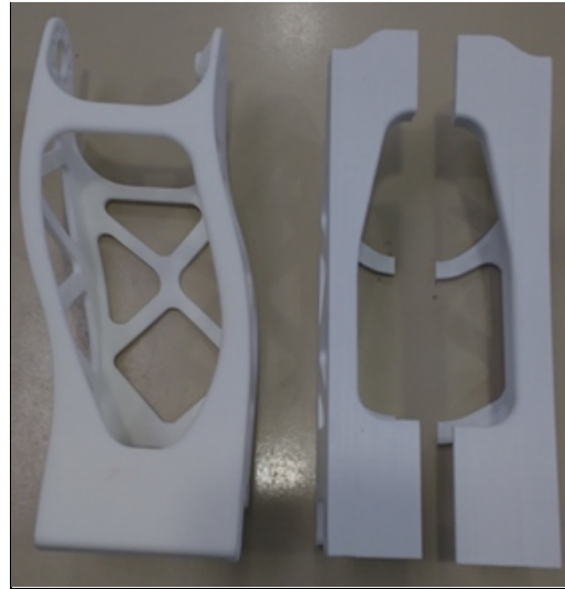
Figure 1.2.1b: The first version of the modified thigh compared to the final thigh design (reproduced as is from Iglesias et al., 2016)
