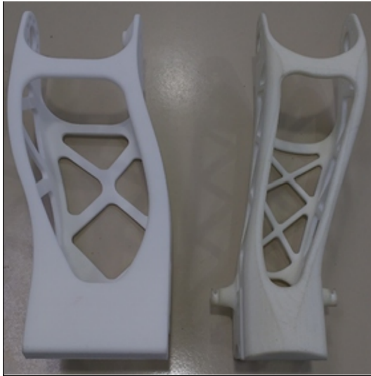
Figure 1.2.1a: The first version of the modified thigh compared to the original Poppy thigh (reproduced as is from Iglesias et al., 2016)
