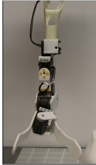
Figure 4.2.7: Actuating hands on a wrist design for Poppy (reproduced from Sosa (2015))
