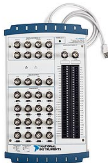
Figure 17: Data acquisition box
