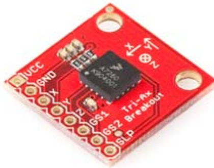
Figure 4-13: Triple Axis Accelerometer MMA7260Q Breakout board
