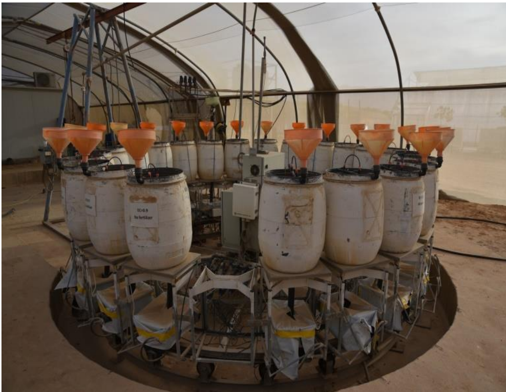
Figure 10: Carousel Irrigation System overview
