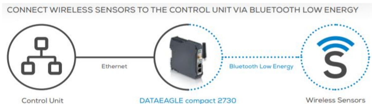
Figure 22: Connect Wireless Sensors to the Control Unit via Bluetooth Low Energy
