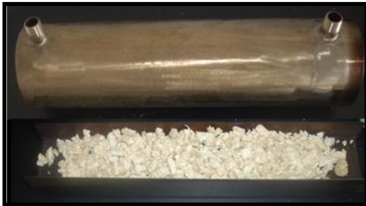
FIGURE 8: REACTOR (TOP) AND SIEVE TRAY FILLED WITH CORNCOB BIOMASS (BOTTOM)
