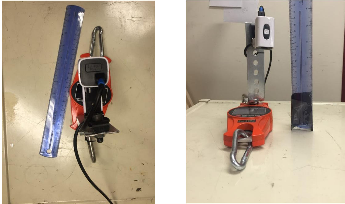
Figure 7: Images of Load Scale with Camera Setup
