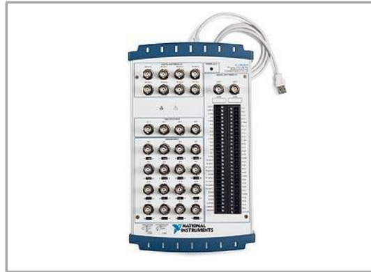
Figure 12: Image of National Instruments TS, USB 6229 BNC Data Acquisition Box from ES3901 Lab Report.
