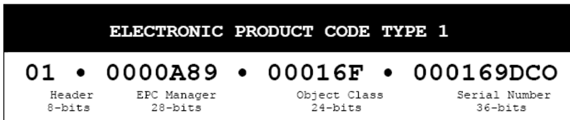
Figure 2: Example of an Electronic Product Code (EPC)
