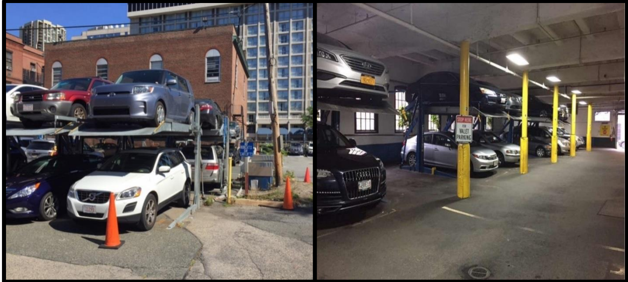
FIGURE 7. Vehicle lifts in the North Anderson Street Lot servicing the Wang Ambulatory Care Center (left). Car stacking machines in use at the Brimmer Street Garage, a single-level residential parking facility (right) (Ian Smith, 2016).
