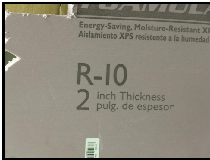
Figure 5 Picture of Insulation with printed R-value and thickness
