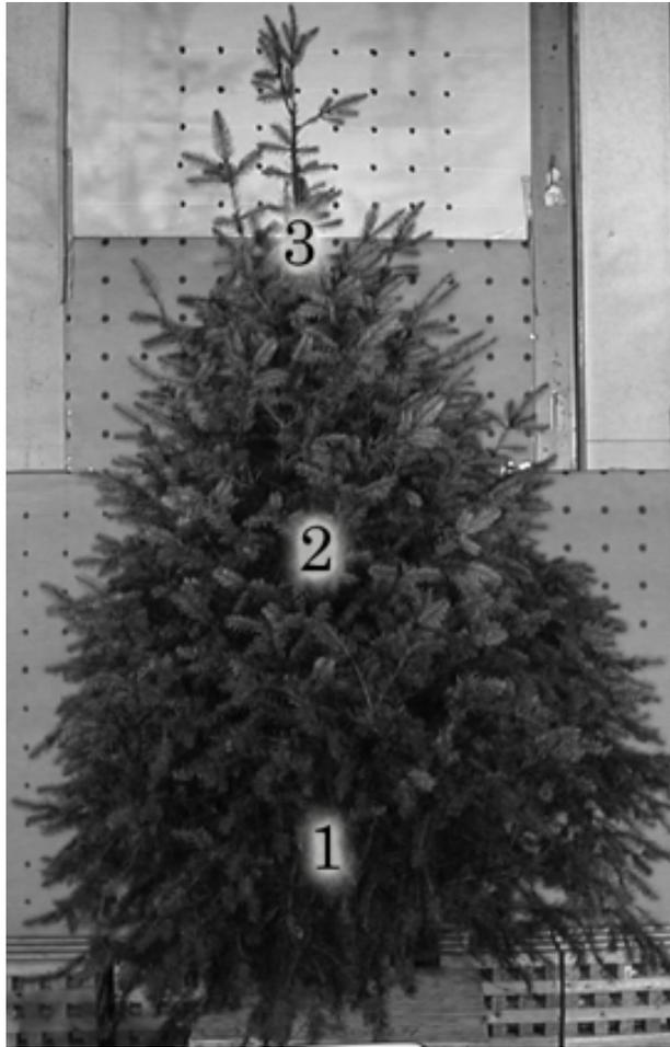
Figure 4.7: Sampling points for the needles taken to measure moisture content are shown here. Samples were taken from the bottom, middle, and top thirds of the tree, labeled as points 1, 2 and 3, from the front and rear faces of the tree.
