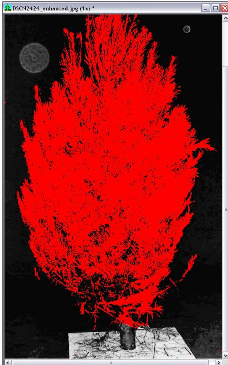
Figure 3.10: A screenshot from the software program used to create and count colored pixel overlays which are used to calculate leaf area. In this example the pixels that meet criteria of color and hue matching those of the needles are highlighted and counted, allowing surface area to be measured for irregular-shaped objects such as trees.
