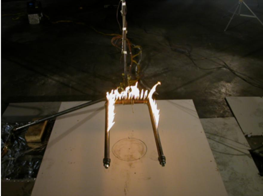
Figure 4.10: Photo of flames, reaching approximately 12 cm high, from the gas burner used to ignite trees.
