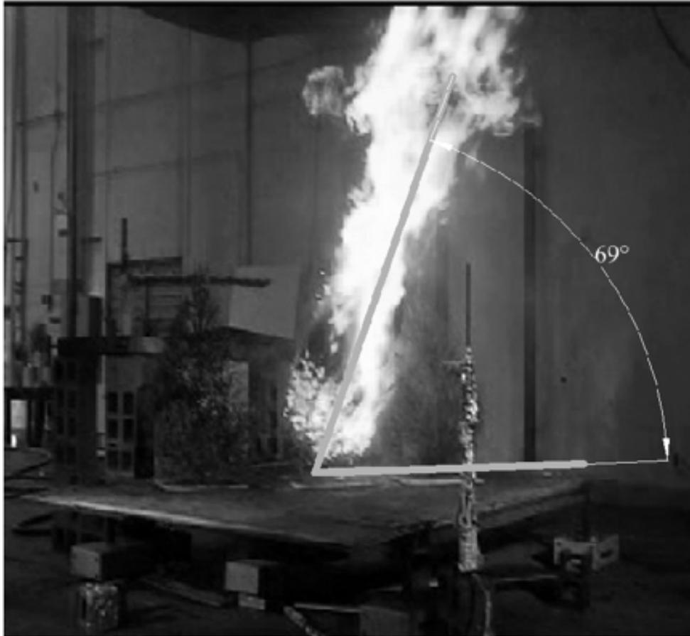
Figure 5.5: Video capture from test 4 showing the flame angle due to wind as flames spread from tree #4 to tree #12.
