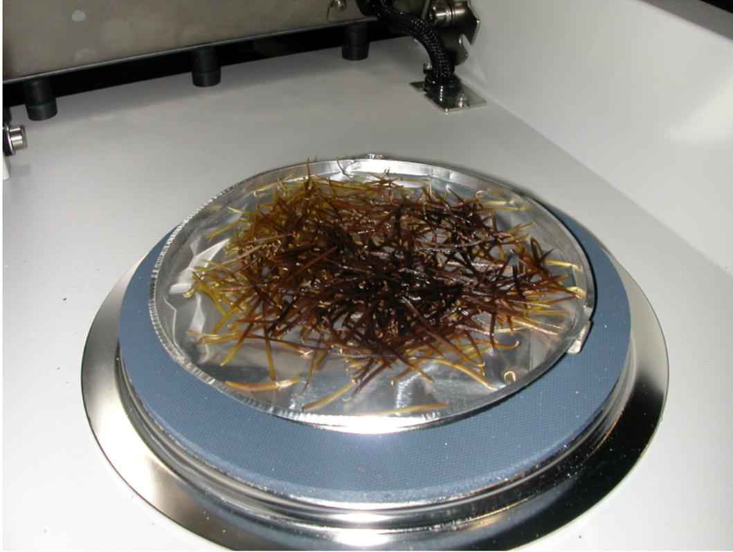
Figure 3.3: A photo of the Computrac Max-1000 sample pan with dehydrated Douglas-fir needles after the moisture content of a sample has been measured.
