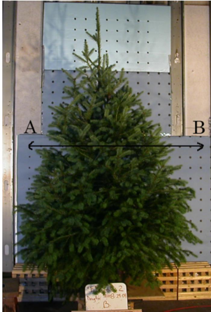
Figure 4.14: Photo a one of the trees prior to being burned in front of the grid backdrop used to calibrate distances in the digital photos for the purpose of measuring the leaf area, where the distance between 'A' and 'B' is known.
