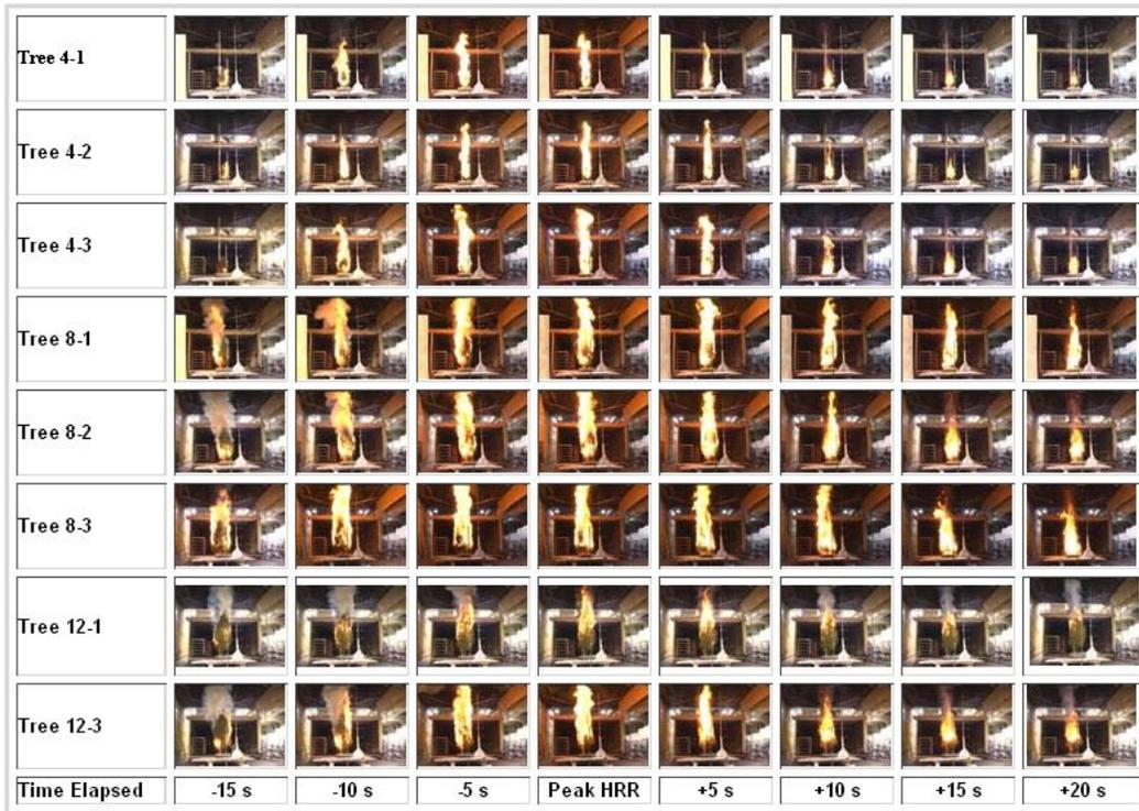
Figure 3.12: Fire video image-captures arranged by 5 second centered around the time of peak HRR showing the progression from ignition to peak is nearly the same time scale in all tree fires regardless of tree size.
