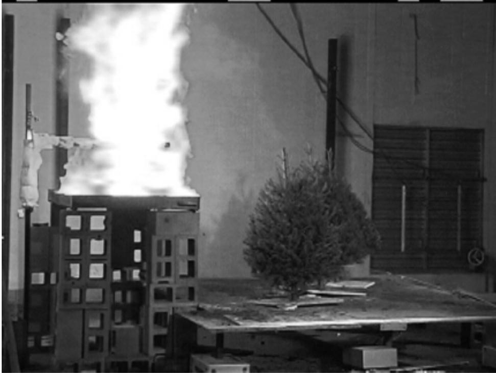
Figure 5.8: Photo of heptane burner heating a cluster of trees as part of fire spread experiments.
