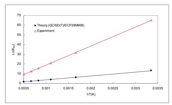
Figure 16: Equilibrium Constant as a Function of Temperature (As + OH → AsO + H)
