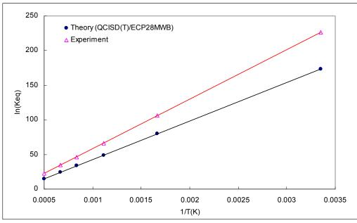
Figure 30: Equilibrium Constant as a Function of Temperature (As +  $O \rightarrow AsO$ )
