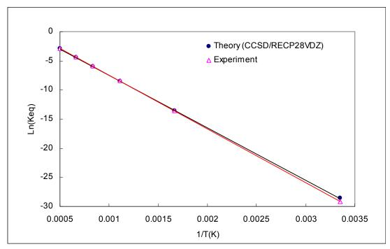
Figure 25: Equilibrium Constant as a Function of Temperature (Se +  $O_2 \rightarrow$  SeO + O)
