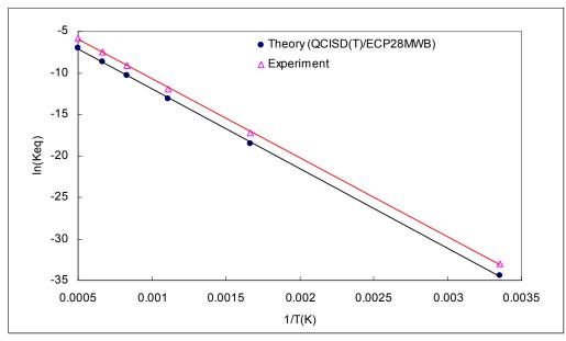
Figure 31: Equilibrium Constant as a Function of Temperature (SeO +  $O_2 \rightarrow SeO_2 + O$ )
