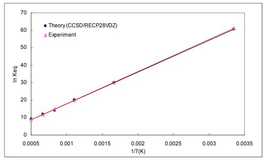
Figure 38: Equilibrium Constant as a Function of Temperature (Se + OCl → SeO + Cl)
