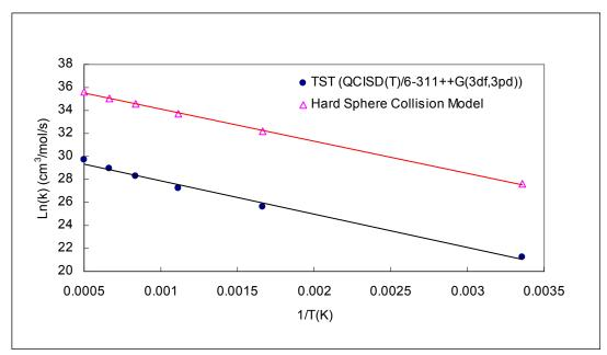
Figure 20: Rate Constant as a Function of Temperature (AsCl + H  $\rightarrow$  As + HCl)
