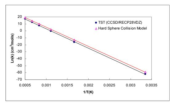
Figure 23: Rate Constant as a Function of Temperature (Se +  $O_2 \rightarrow SeO + O$ )
