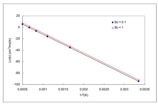
Figure 28: Rate Constant as a Function of Temperature (SeH<sub>2</sub>  $\rightarrow$  Se + H<sub>2</sub>/Ar bath gas)
