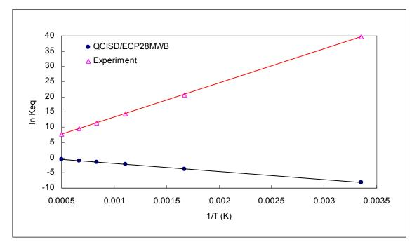
Figure 11: Equilibrium Constant as a Function of Temperature (As +  $O_2 \rightarrow AsO + O$ )
