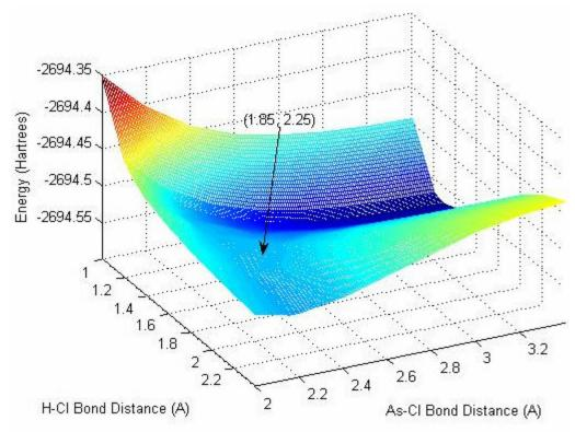
Figure 17: As + HCl  $\rightarrow$  AsCl + H (PES)
