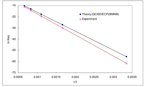
Figure 32: Equilibrium Constant as a Function of Temperature (As + OH  $\rightarrow$  AsH + O)
