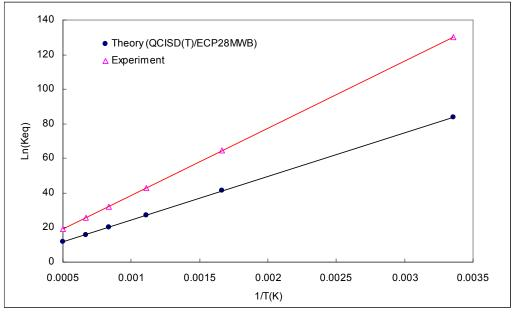
Figure 34: Equilibrium Constant as a Function of Temperature (As + OCl → AsO + Cl)
