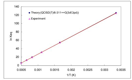
Figure 36: Equilibrium Constant as a Function of Temperature (Se +  $O_2 \rightarrow SeO_2$ )
