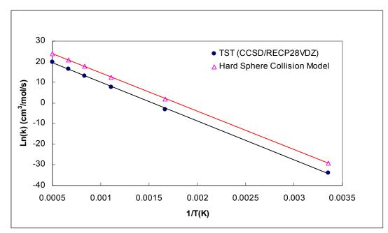
Figure 24: Rate Constant as a Function of Temperature (SeO + O  $\rightarrow$  Se + O<sub>2</sub>)
