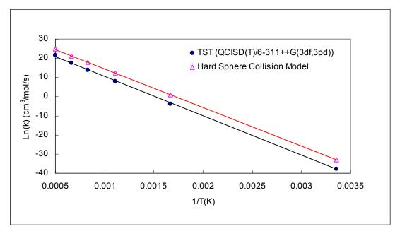
Figure 19: Rate Constant as a Function of Temperature (As + HCl → AsCl + H)
