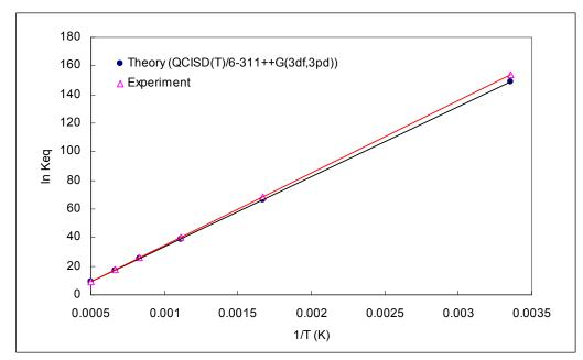
Figure 37: Equilibrium Constant as a Function of Temperature (SeO + O  $\rightarrow$  SeO<sub>2</sub>)
