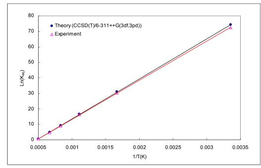
Figure 29: Equilibrium Constant as a Function of Temperature (Se +  $H_2 \rightarrow SeH_2$ )
