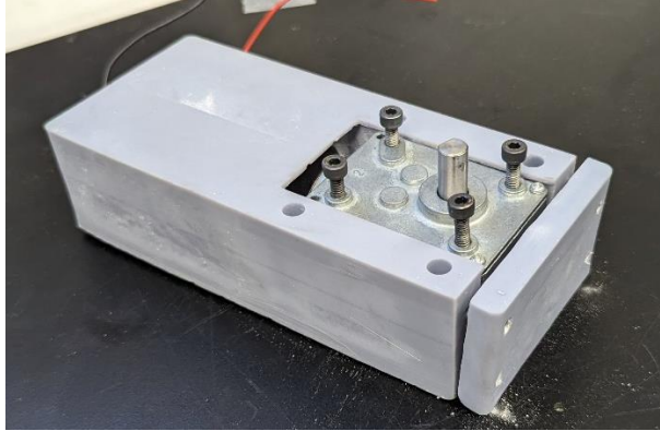
Figure 20: Assembly of the net release motor prior to chemical welding and sealing.
