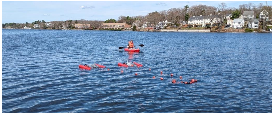
Figure 38: Tandem robot operation during Lake Quinsigamond open water test.
