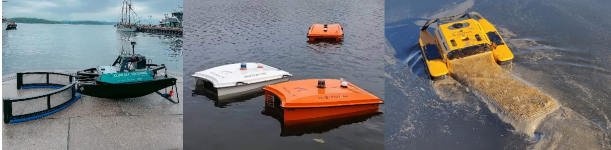
Figure 7: (Left) Clean Sea Solution's Aquadrone ready for deployment in Oslo [14]. (Middle) Three Wasteshark systems collecting trash in an urban river [52]. (Right) Jellyfishbot with a full net of reclaimed waste [31].
