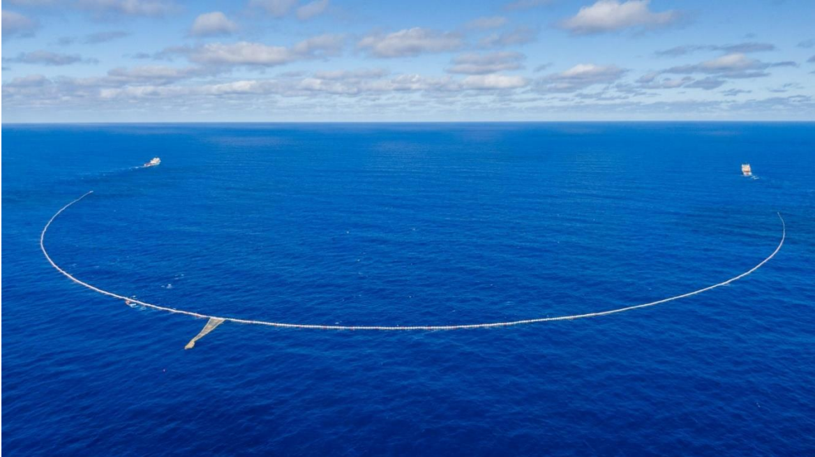
Figure 2: An aerial shot of The Ocean Cleanup's System 03 collecting waste in the Great Pacific Garbage Patch halfway between Hawaii and California [35].
