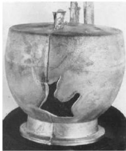
**Figure 2.7 Misrun defect**
