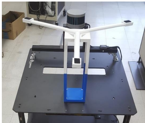
Figure 9: Fully-Printed Sensor Stand.
