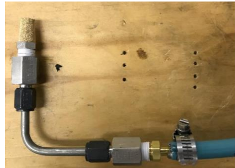
Figure 15: 2019 MQP Diffuser (Point Source Sparger).
