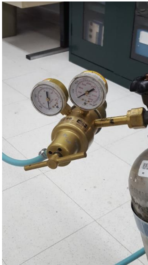
Figure 12: Harris® Model 9296 Regulator that will generate the plume.
