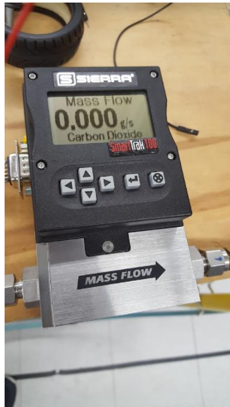
Figure 13: Sierra© SmartTrak C100L Mass Flow Rate Meter.
