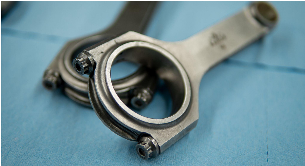
Figure X: ARP 2000 Rod Bolts (mock installation without crankshaft for reference)
