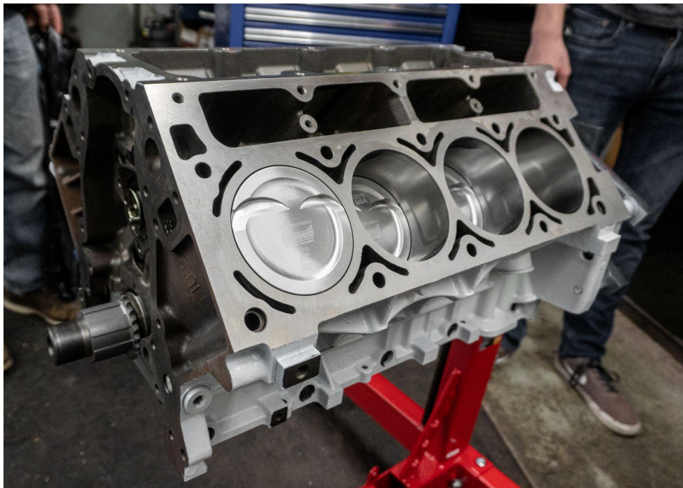
Figure X: Engine block after installation of crankshaft, camshaft, piston and rod assemblies
