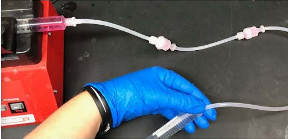
Figure 5.8 Setup of Filtration with Pump for 1 \mu\text{m} and 10 \mu\text{m} Filter in Series
