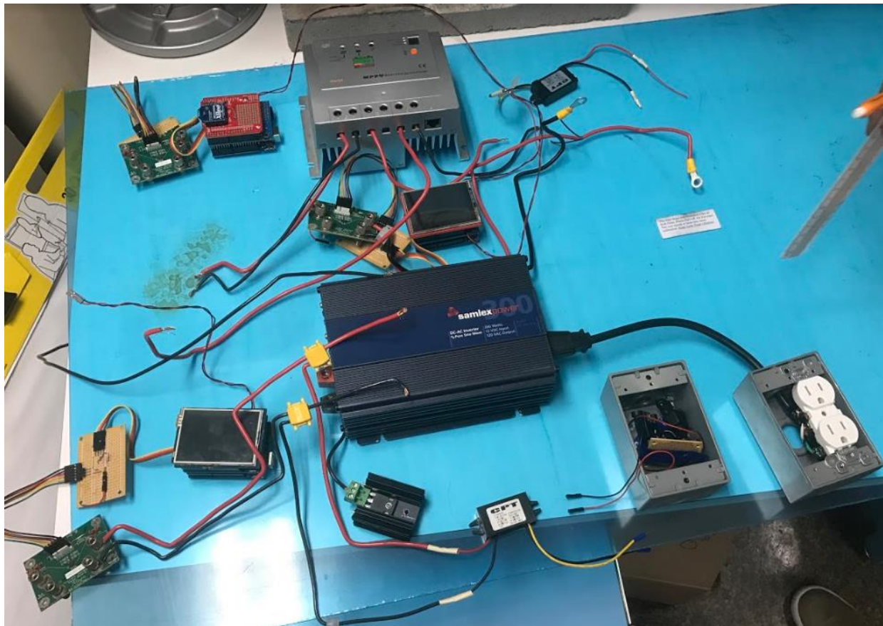
Figure 27. Solar Charging Station removed from the wooden board
