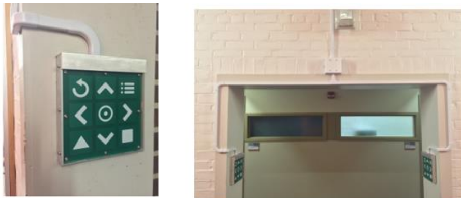
Figure 7. Capacitive Touch Sensor mounted in doorway
