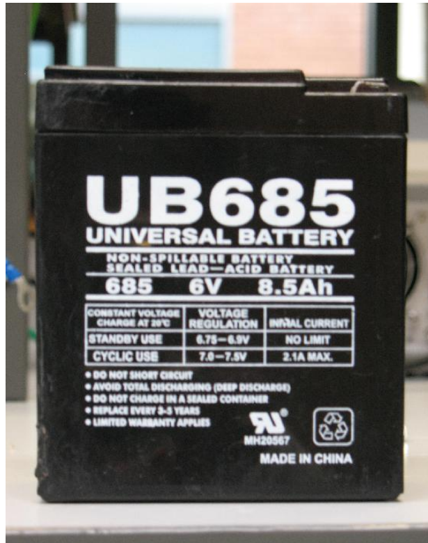
Figure 10: 6V sealed lead acid battery.
