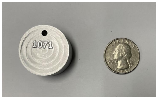
Figure 44 FNC sample after machining and cleaning
