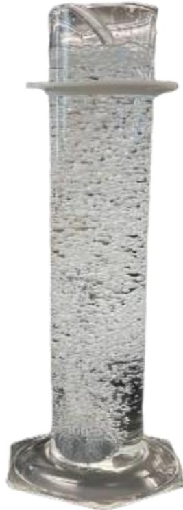
Figure 4. This image is an example of a foam or bubble fractionation bubbler. If a stable foam forms on top of the column, it would be considered foam fractionation. If a stable foam does not form, then it would be considered bubble fractionation.
