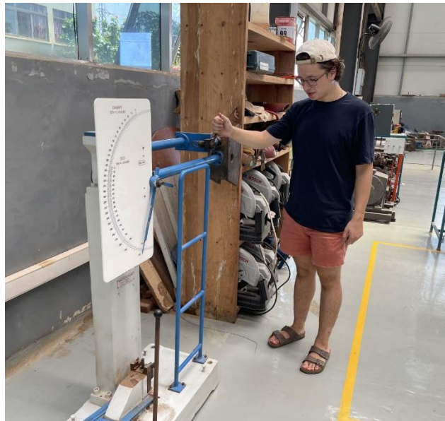
Figure 26: Photo of Mike performing the impact test. Photo Credit: Abu Karim
