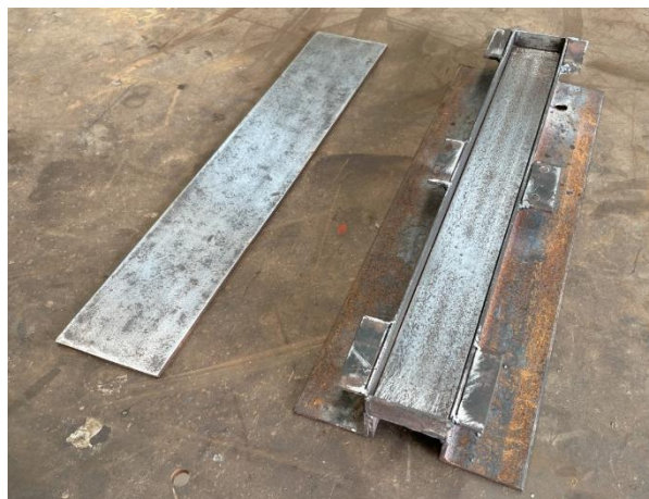
Figure 11: Photo of the final welded and polished mold assembly. Photo Credit: Michael Morin
