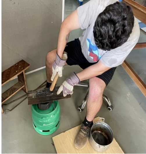
Figure 16: Photo of Jack spreading the LDPE melt into the heated mold. Photo Credit: Michael Morin
