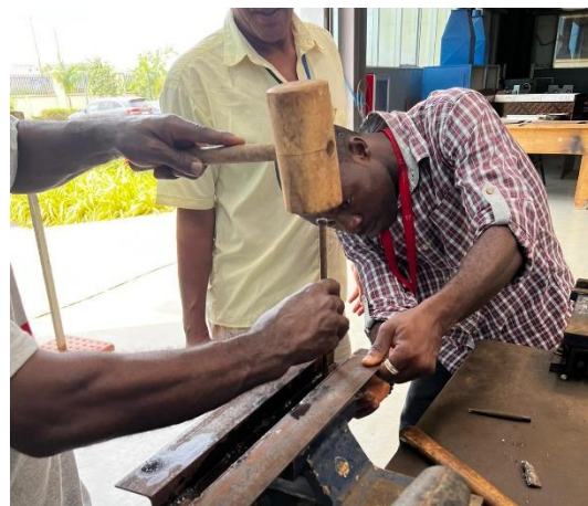
Figure 19: Photo of Ben using a mallet and tap in attempt to remove the bar with assistance from Abu. Photo Credit: Jackson Baker
