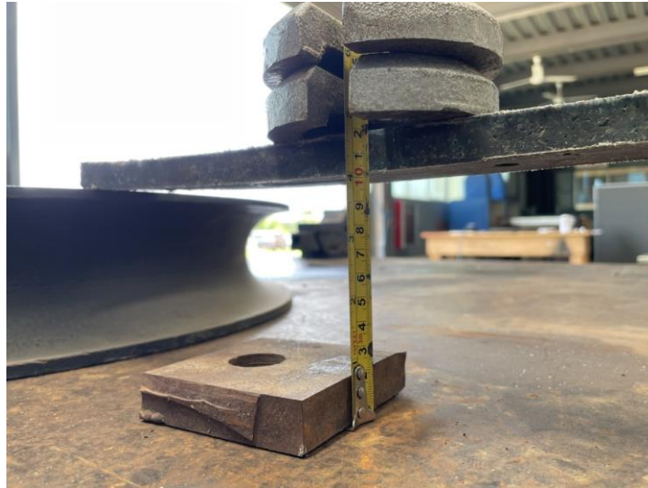
Figure 23: Photo of the three-point deflection test set-up for 2kgs. Photo Credit: Michael Morin
