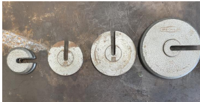
Figure 13: Photo of the 1kg, 2kg, 4kg, and 10kg standard weights for deflection testing. Photo Credit: Michael Morin
