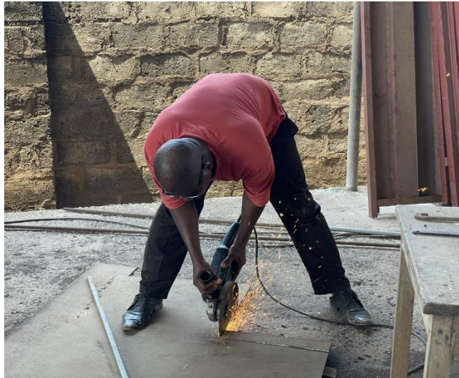
Figure 9: Photo of local scrap yard owner cutting the lid piece from a large sheet of mild steel. Photo Credit: Michael Morin
