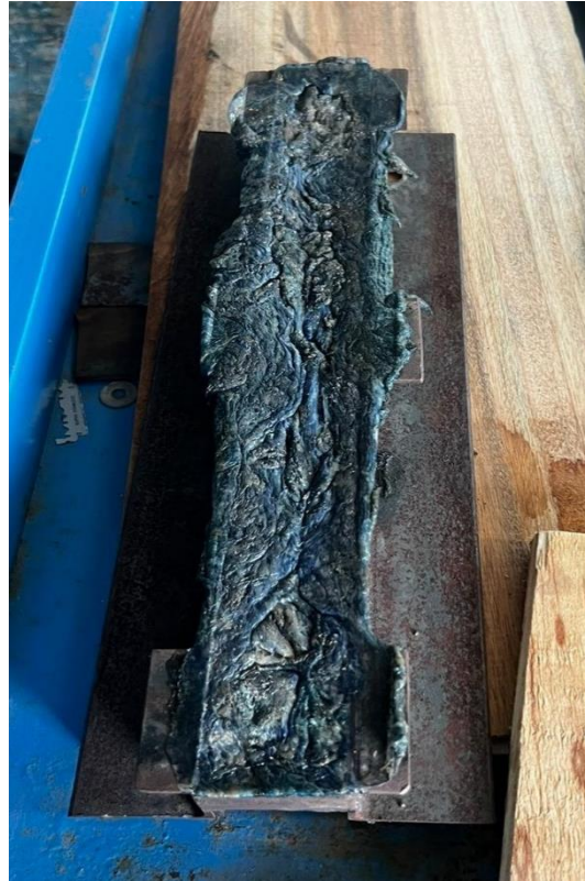
Figure 18: Photo of the resultant LDPE bar in the cooled mold. Photo Credit: Jackson Baker
