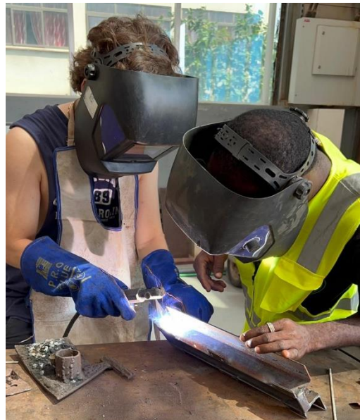
Figure 10: Photo of Mike welding the clamp pads onto the mold with assistance from Abu. Photo Credit: Jackson Baker
