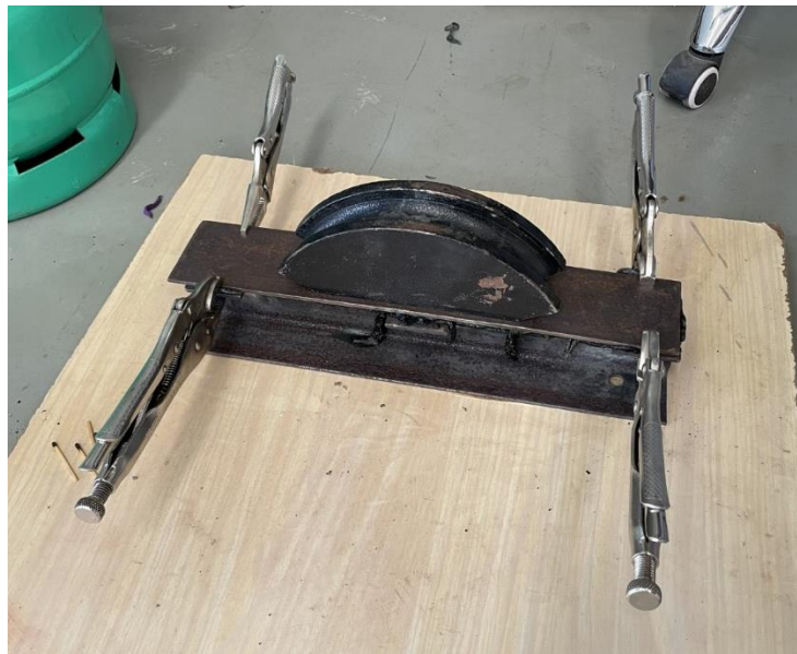
Figure 17: Photo of the melt being compressed into the mold via four hand clamps and a weight. Photo Credit: Michael Morin
