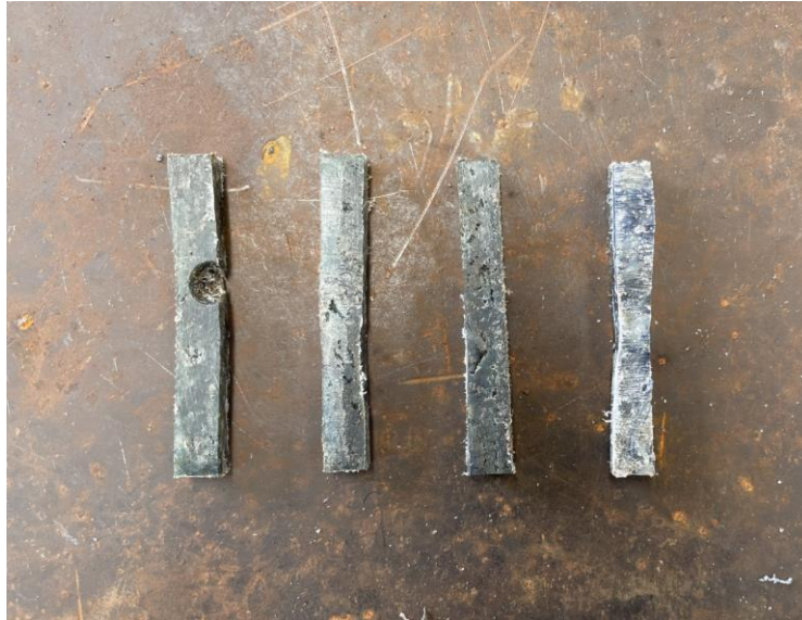
Figure 25: Photo of the four test samples cut from the bar for the Charpy impact test. Photo Credit: Michael Morin
