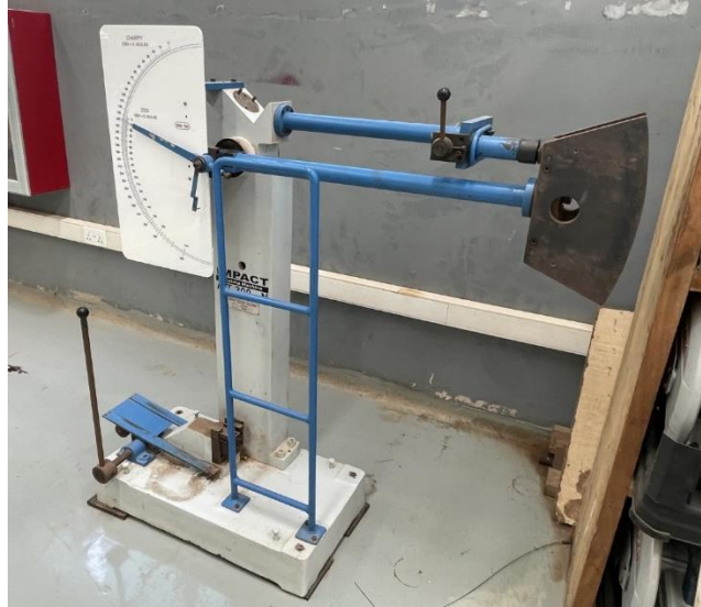
Figure 14: Photo of the AIT-300-N Impact Testing Machine. Photo Credit: Michael Morin
