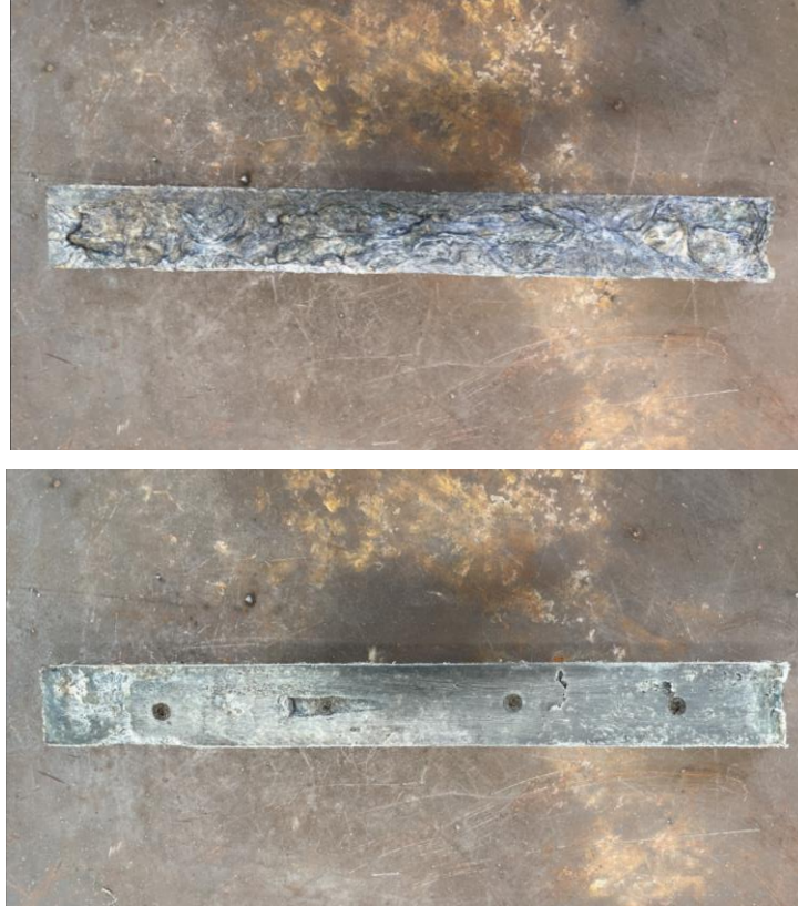
Figure 22: Photos of the top of the bar (top) and the bottom of the bar (bottom). The top is notably rough and wavy, and the bottom is smooth with demolding damage. Photo Credit: Michael Morin
