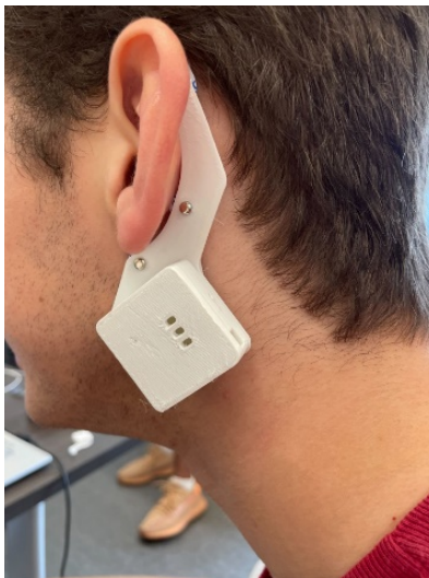
Figure 33 Final top half with bumps, changed contact location, increased thickness, and adjusted bump shape
