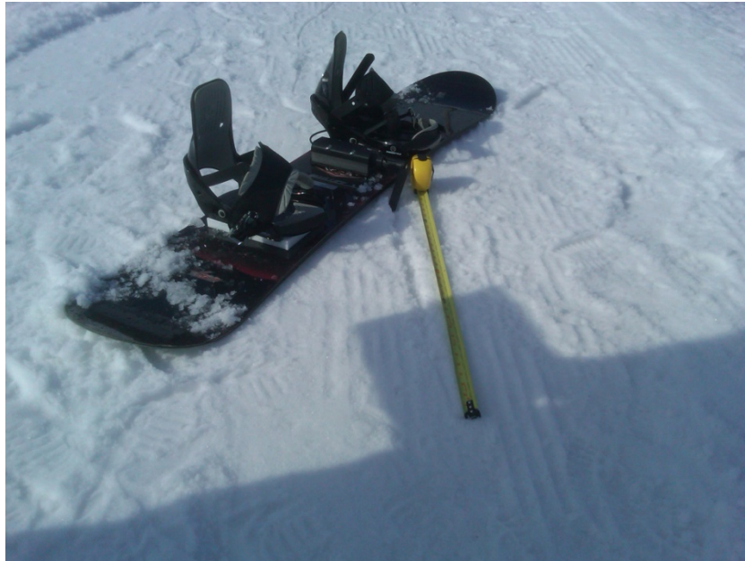
Figure 4.2: The result from a parallel static test on a 10 degree slope on groomed snow.
