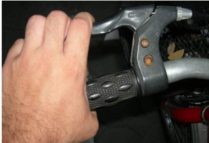
Figure 28: Example of Brake Layout that Could be Used on the New Trolley
