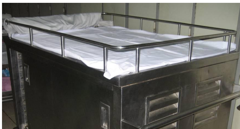
Figure 23: Containment Rack on a Current Trolley
