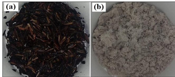
Figure 2.6. a) RHA burned at 300 °C (572 °F). b) RHA burned at 650 °C (1202 °F)
