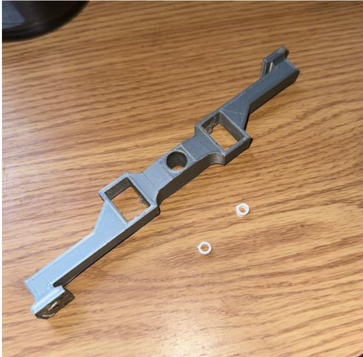
Figure 26: 3D Print of “New Lever Arm 1.0” and Spacers from “Clamp Flanges 1.0” Print
