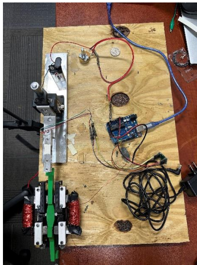
Figure 48: Original Strain Gage Setup
