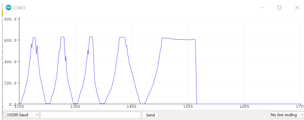
Figure 60: Force vs. Time Graph for Four Degree Deflection Angle
