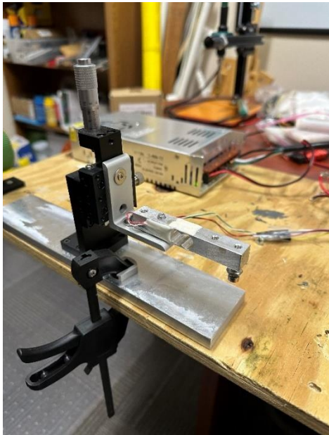
Figure 70: Clamping the Strain Gage
