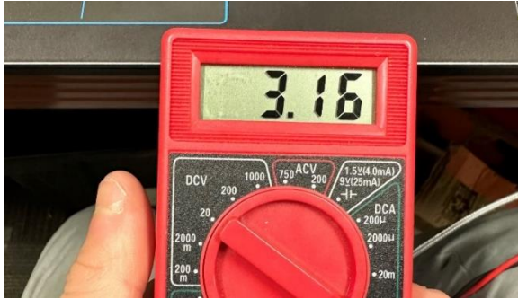
Figure 68: Maximum Current Output from Voltage Regulator
