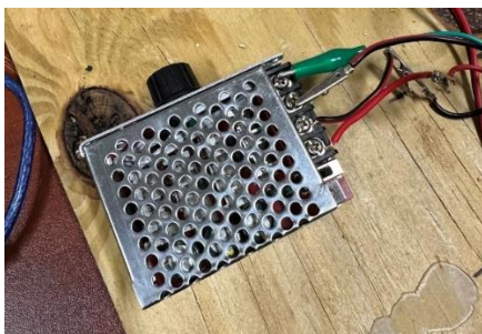
Figure 67: Voltage Regulator in Strain Gage Circuit
