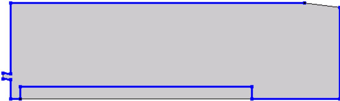
Fig. 39. Boundary conditions chosen as wall functions (blue lines) in COMSOL
