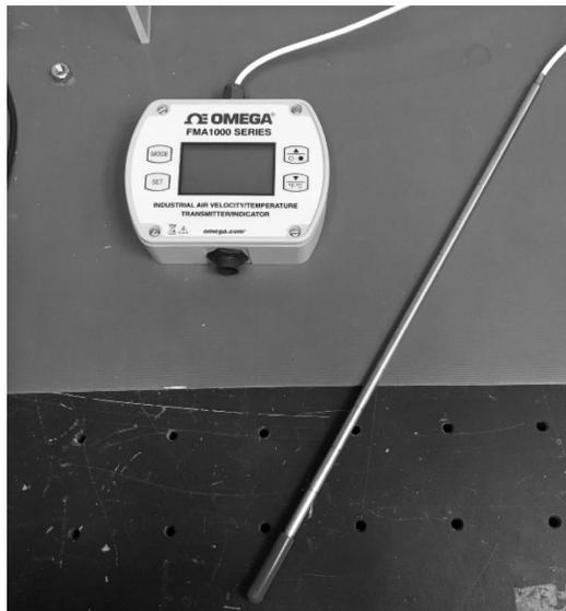
Fig. 22. Omega FMA1000-R V1 air velocity/temperature transmitter
