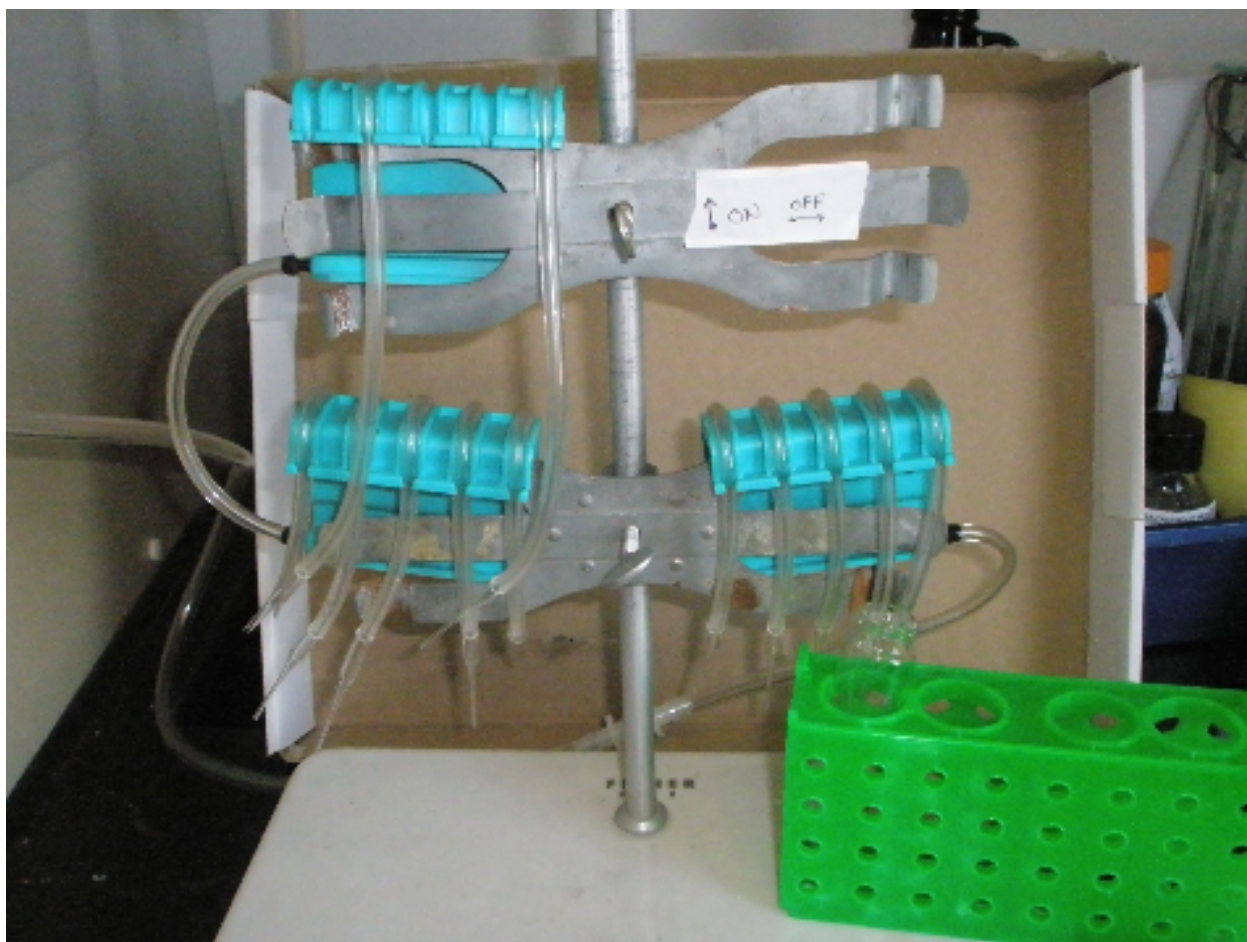
Figure 8: Assembled nitrogen gas drying apparatus
