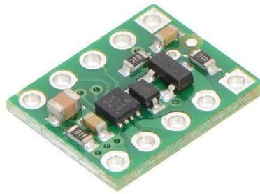
*Figure 46: DRV 8838 Single Motor Driver Carrier*
