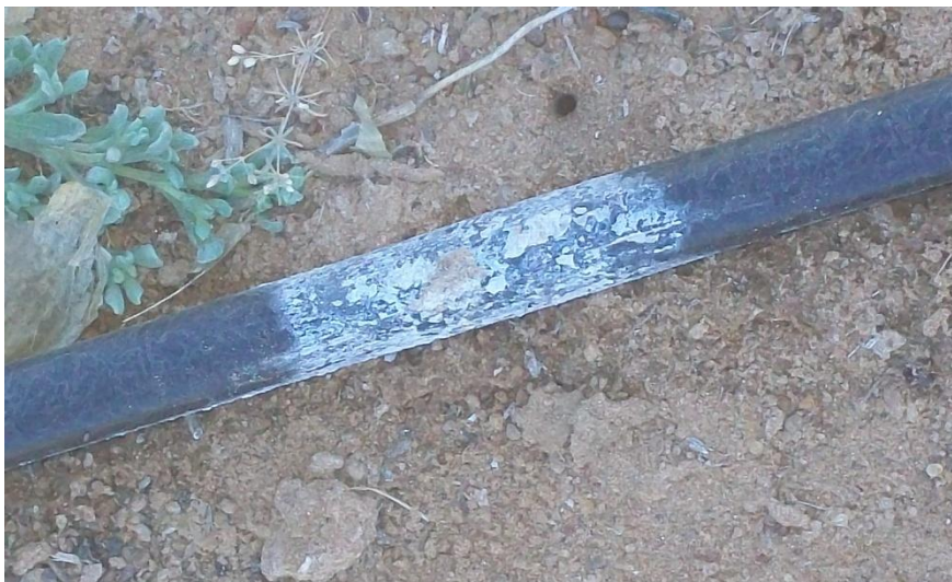
Figure 25- Calcium deposit on an irrigation pipe in Drimiopsis
