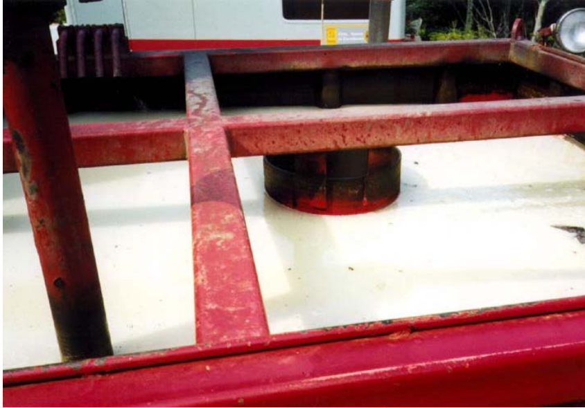
Figure 3.5: Gelled water is pre-mixed in a truck-mounted mixing tank. Photograph shows a batch of linear, guar-based gel. This gel is used to transport the sand proppant into the fracture propagated by the nitrogen foam treatment. lxiv
