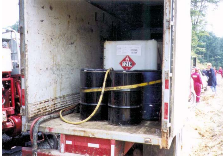
Figure 3.3: Chemicals are stored on site in a support truck. Fracturing fluid additives such as the foaming agent can be pumped directly from storage containers to mix tanks. xxxiii
