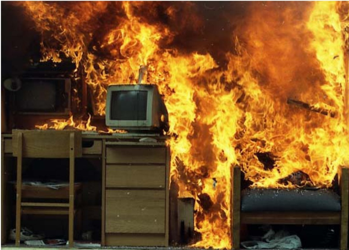
Figure 13 The fire spread rapidly until it reached the ceiling tapestry. At that point, it then spread quickly horizontally until the burning tapestry fell down onto the other combustibles in the room.
