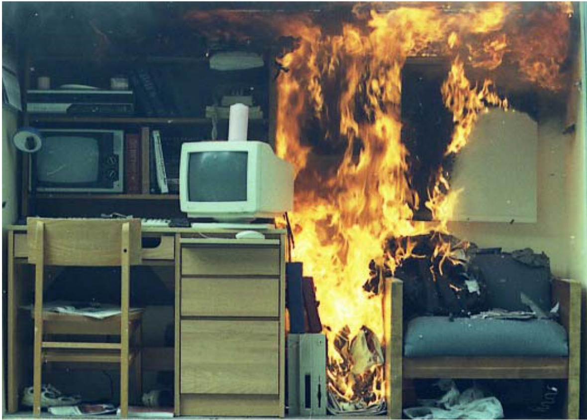
Figure 12 This burn started in a trash can located between the desk and the chair. There is plenty of fuel and a continuous vertical fuel path for the fire to travel.
