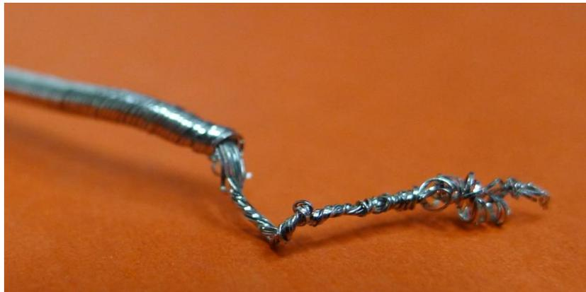
Fig. 2.8. Torque coil failed during the rotation test shown in Fig. 2.4. The failure occurs at the connection with the motor.
