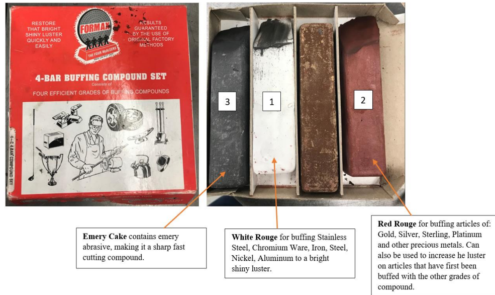
Figure 29. Buffing Compound Set for Polishing SS Plates © 2019 Formax Manufacturing
