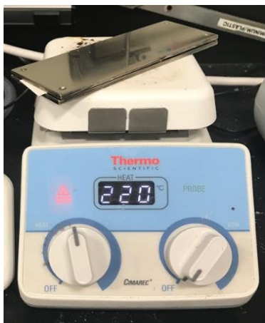
Figure 30. Flattening the ABS Strip
