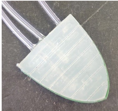
Figure 29: Image of rear entrance design prototype
