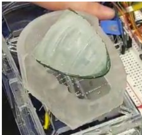
Figure 66: One of several tongues with burst interior channels.
