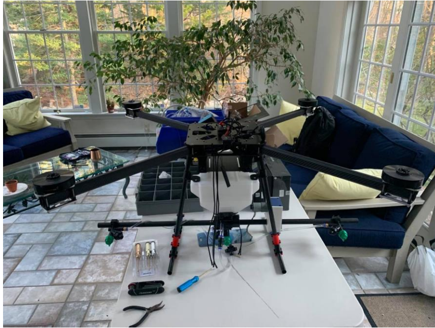
Figure 21. Fully assembled landing gear mounted to the drone center frame
