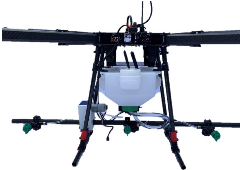
Figure 24. Close-up of spray-bar on the built drone
