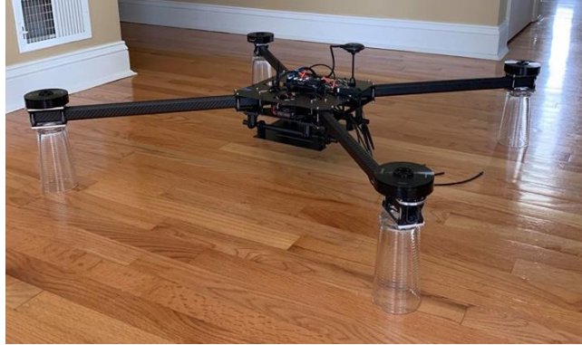
Figure 33. Leveling the Drone
