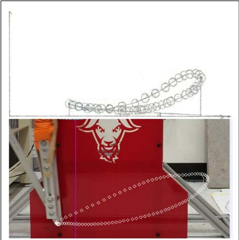
Figure 76: Trace curve of ankle. (Top) OpenSim trace curve (Bottom) Prototype trace curve
