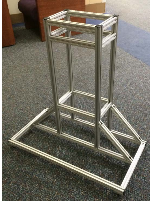
Figure 55: The Assembled 80/20 Component of the Frame.
