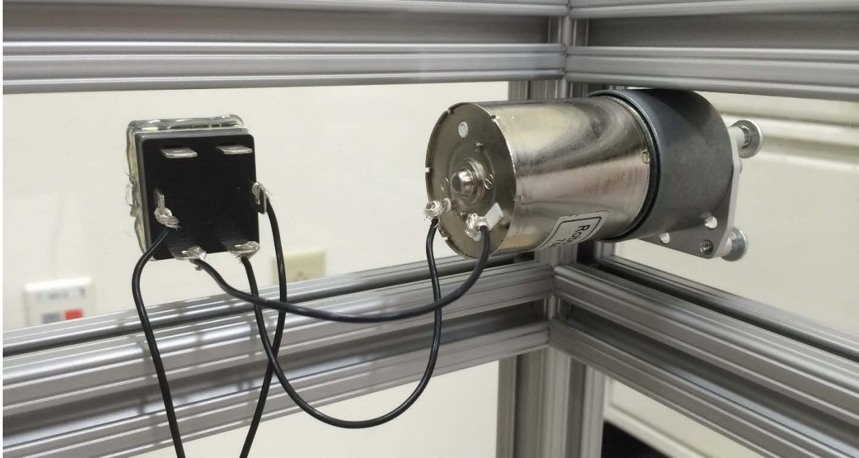
Figure 59: The Motor and Switch Mounted to the Frame and Wired Together
