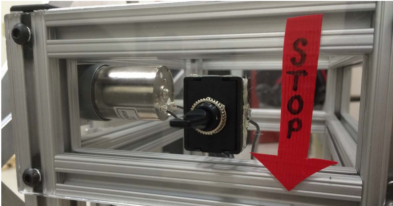
Figure 57: The Switch is Hot-Glued into the Rectangular Cutout in the Side Acrylic Plate with the Stop Label to its Right
