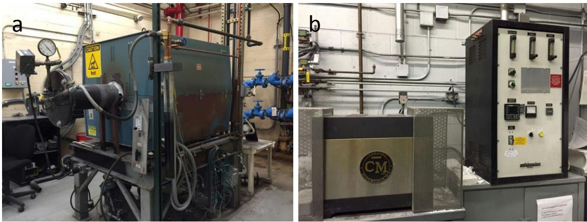
Figure 25: Two pictures of a) the tube furnace and b) the CM conditioning furnace.
