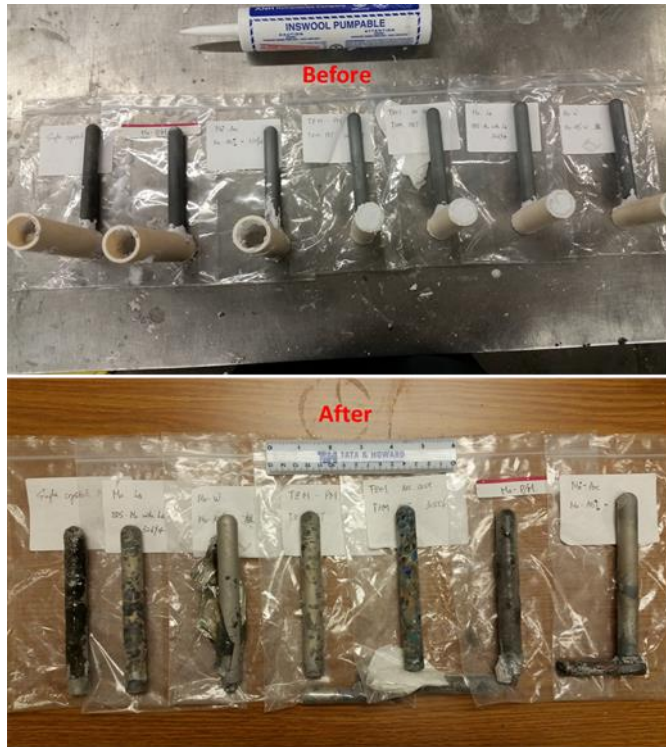
Figure 72: The picture of the coated electrodes before and after the corrosion test in borosilicate glass.
