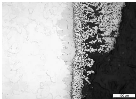
Figure 22: Cross-section of the metal-glass interface of sample after 168 hours in opal glass(87).
