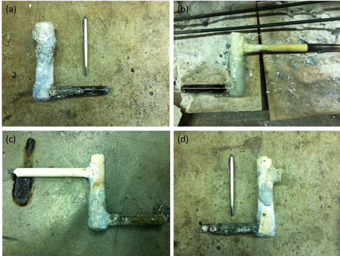
Figure 52: The pictures of the molybdenum electrodes after the first corrosion test, (a) coated sample without AC, (b) coated sample with AC, (c) uncoated sample with AC, and (d) uncoated sample without AC. There were more yellow deposits observed on uncoated electrodes than on coated ones. Also more yellow deposits were observed on the uncoated electrode with AC than the uncoated electrode without AC.
