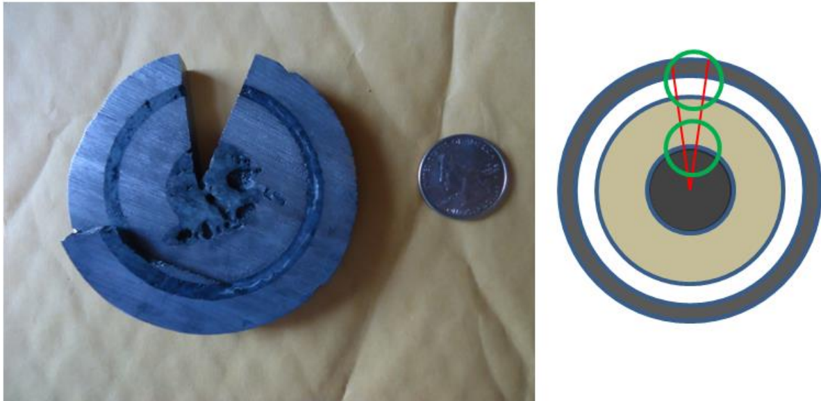
Figure 8: Two metallurgical samples were prepared from the green circle position.
