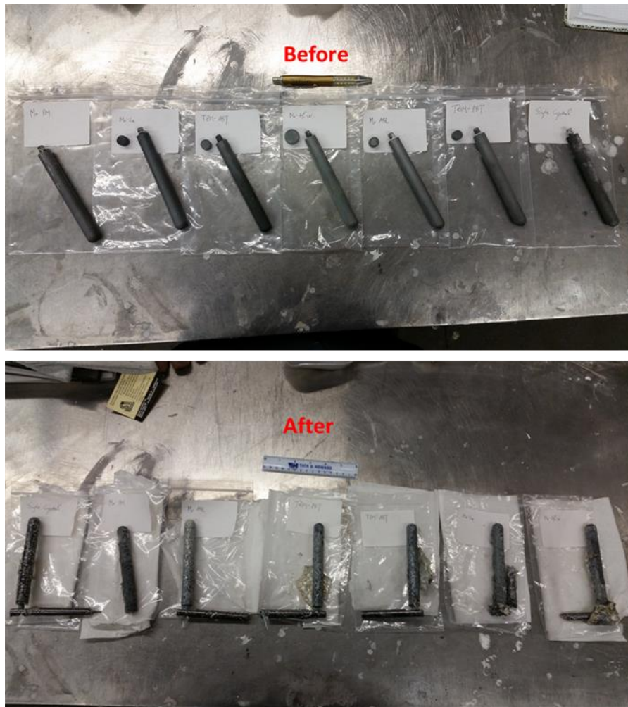
Figure 65: The picture of the coated electrodes before and after the corrosion test in soda-lime glass.
