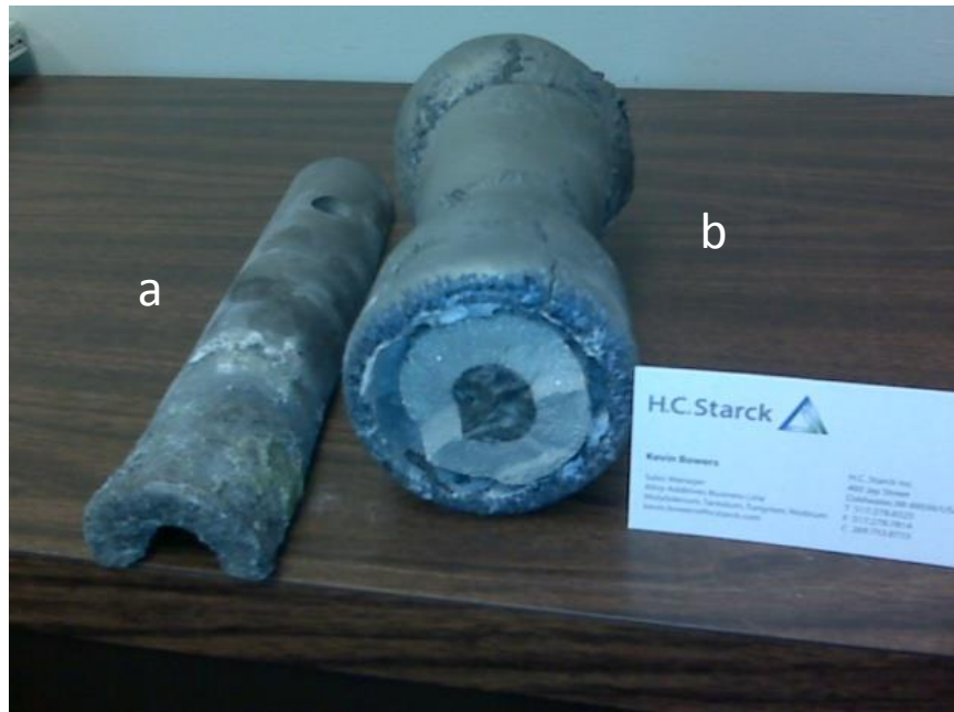
Figure 4: Molybdenum electrode assembly: a) electrode head, and b) electrode shaft.
