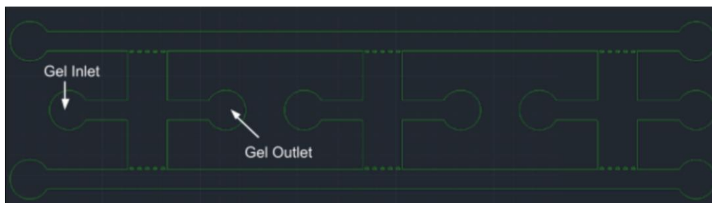
Figure 10: AutoCAD Design 1. Design 1 has a gel inlet and outlet for each of the three gel chambers, which sit between the fluid channels are 1 mm by 3 mm. The fluid channels on the top and bottom of the device are 17 mm in length.
