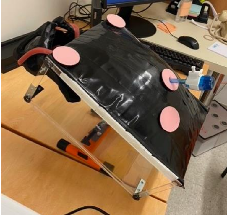
Figure 57. Final prototype of gynecological laparoscopic trainer.
