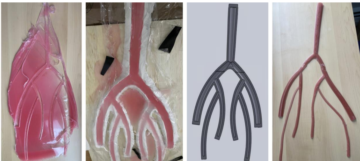
Figure 46. Three molds used in the vessel network silicone molding process of creating the vessel network; silicone mold (left), clay mold (middle left), 3D print PLA mold (middle right), and final vessel network phantom (right).
