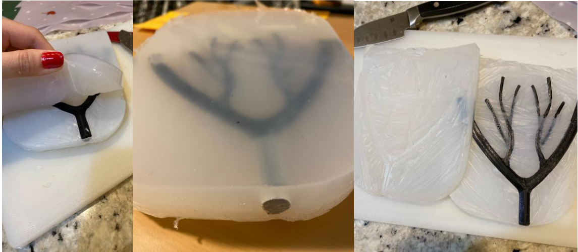
Figure 42. Silicone molding process for creating a vessel network mold.
