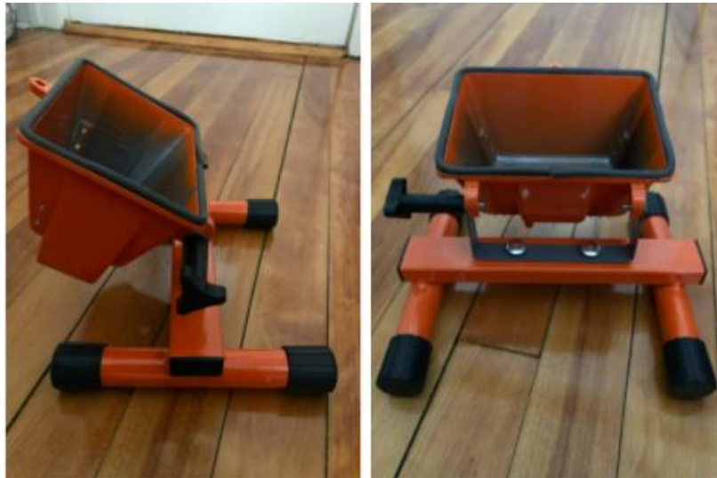
Figure 37. Modified adjustable light fixture for the rotational mechanism of abdominal casing box.
