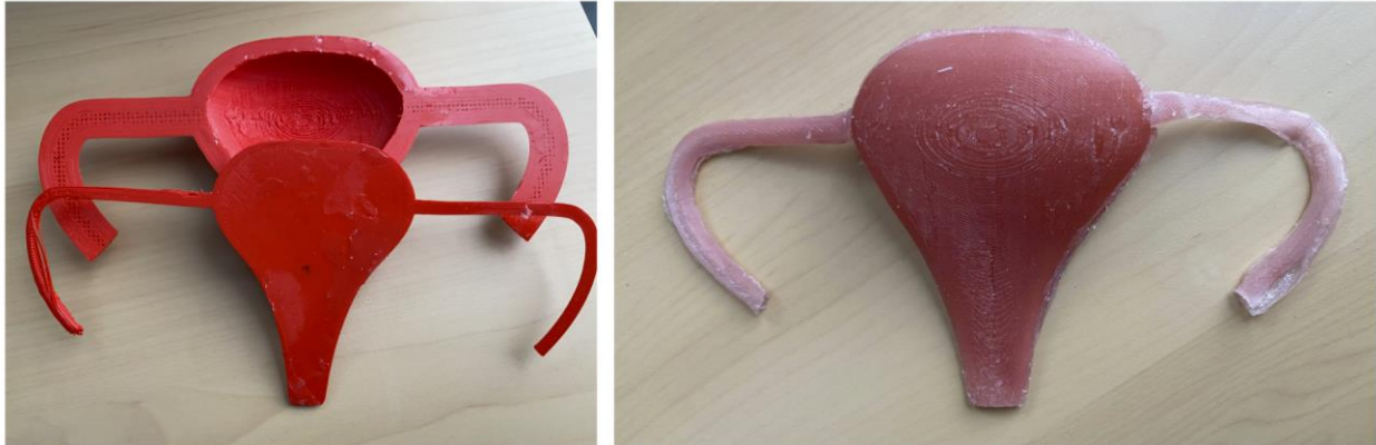
Figure 52. Final uterus 3D printed PLA parts (left) and final silicone uterus phantom (right).
