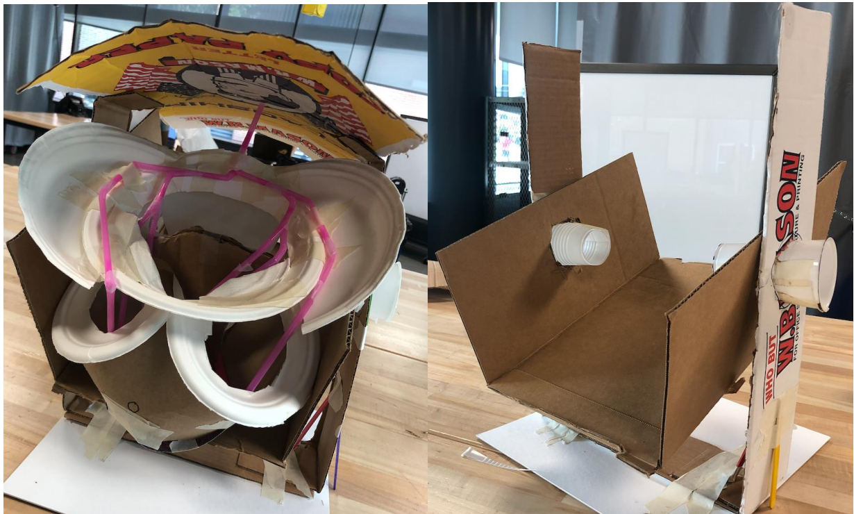
Figure 18. Pelvis mock-up in abdominal casing (left) and rotational mechanism of mock-up (right).
