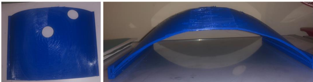
Figure 34. Final abdominal casing top PLA print.
