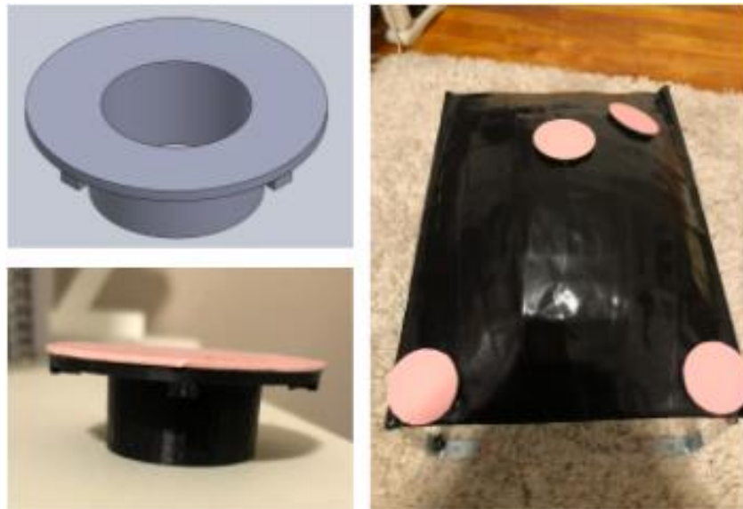
Figure 36. Abdominal casing inserts for instruments. CAD model of insert part (top left), 3D printed model with silicone top (bottom left), and parts inserted into top curve (right).
