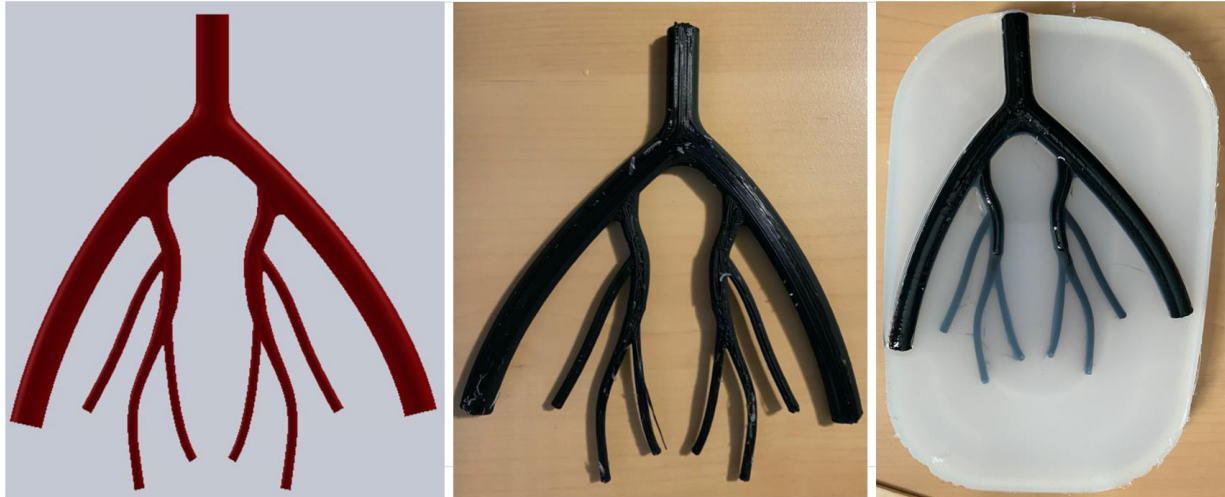
Figure 41. Vessel network CAD model (left), 3D printed PLA vessel network (middle), and vessel network in silicone molding process (right).
