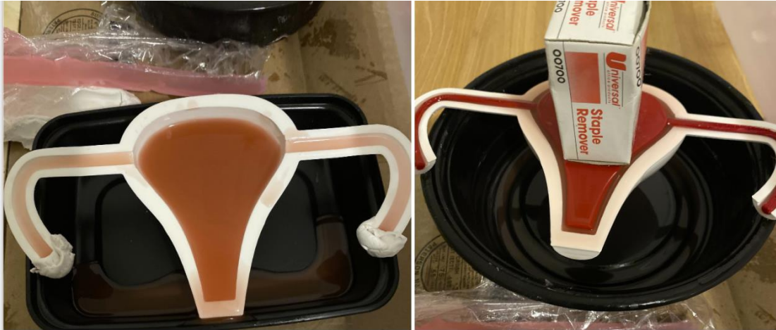
Figure 50. Silicone molding process for creating half of the uterus phantom.
