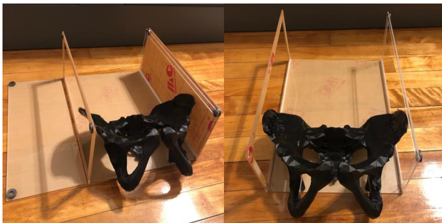
Figure 32. Abdominal casing box with pelvic model placed inside. Removable walls with magnets shown (left). Sidewalls removed (right).
